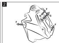
Remove all remaining radiator (F) and seat (G) screws. Close the petcock and disconnect the fuel line from the carb. Remove the original tank.
