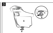
Install the petcock (B) onto the Acerbis Fuel tank (A) using the supplied screws (C) as indicated in the image.
