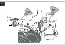
Connect the Fuel line (D) to the petcock and carburetor. If needed use a small dab of 2 stroke oil/pre mix to lube the ends of the fuel line to help install. Tighten hose clamps (E) around the ends of the petcock and Carb.
