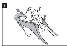
Remove the radiator shrouds and seat from the original tank.
